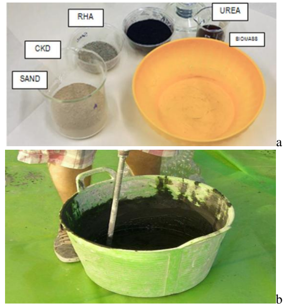
Fig. 3. The main components of the eco-cement product (a) and mixture preparation (b)
