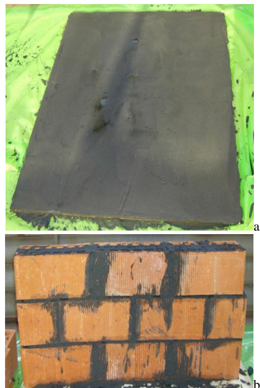
Fig. 4. The plaster layer (a) and wall bricks (b) constructed with the eco-cement mixture
